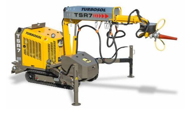
Turbosol TSR-7 is a tracked unit for spraying concrete. It is ideal for underground works or areas difficult to reach. TSR-7 is the best means to move around Safely in rugged and irregular work sites with total autonomy of movement.
