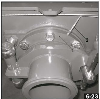
Fix the delivery flange 1 (FIG. 6-23) by tightening the six bolts with 30 mm key.
