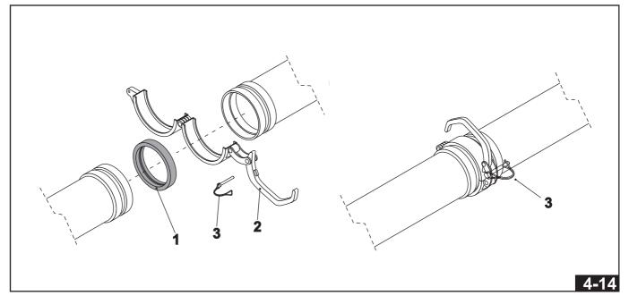
Connect the mortar conveyor piping 1 (Fig. 4-15).
