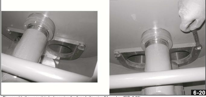
Disassemble the wear plate by loosening the three bolts using 24 mm key (FIG. 6-20)
