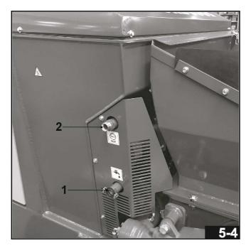
Connect the water intake pipe to the supply fitting 1 (FIG.5-4). Connect the high pressure delivery pipe to the fitting 2 (FIG.5-4).
